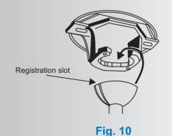
Step 8. Slip the coupling cover, canopy cover and canopy onto the downrod.
